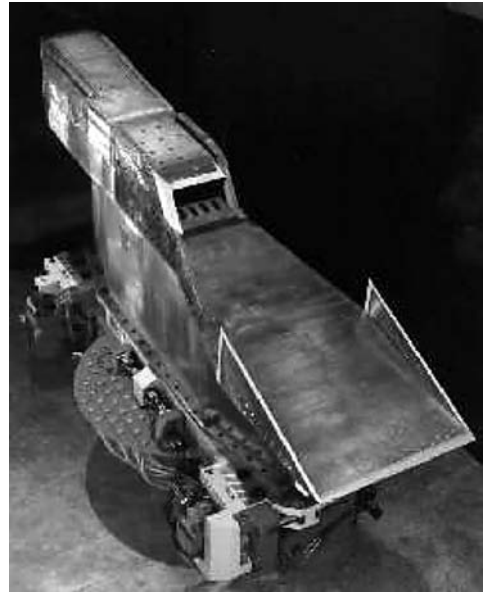
Figure 1.5. The rectangular engine configuration used for the National Aerospace Plane Program's concept demonstration engine mounted atop its pedestal and the six-component force measurement system in preparation for testing in NASA Langley's 8-ft. high-temperature tunnel.
